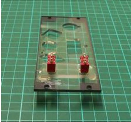
The neck of the switches should fit neatly into the holes already drilled in the supplied panel backplate. Glue the switch plates onto the backplate with hot glue. Any cabling can be soldered directly onto the rear switch terminals.
