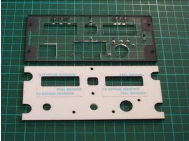
Use very thin double sided tape to stick the cellophane in place. You should be able to get this tape at office stationary stores. Don't use the foam style double sided mounting tape, it's far too thick.
