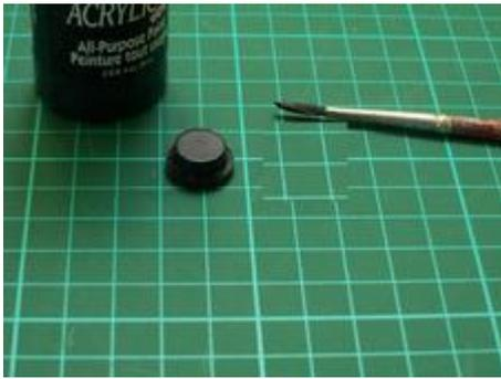
Edges need to be painted black to avoid light leakage when backlit. Use acrylic paint available from any craft shop.
