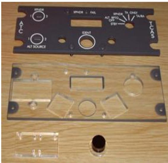
The XPDR panel comprises a front plate laser cut and ready for backlighting, backplate, switch mounting plate and IDENT button.
