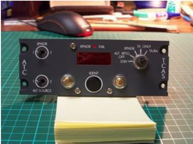
The digital displays look more aesthetically appealing with a coloured lens over them. I used standard red cellophane sandwiched between the front and back plates and it works well.
