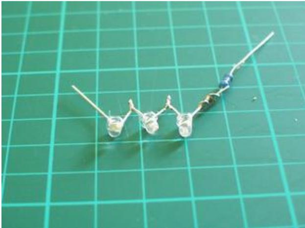
I'm driving my backlighting from a 12v DC power supply and connecting them in a series configuration. The maximum number of these LED's that can be driven from 12v in series is 3, so most of my LED's are grouped this way along with a resistor. These LED's have a working voltage of 3.4v and current draw of 20mA which results in a resistor requirement of 100 ohms per 3 LED's.
