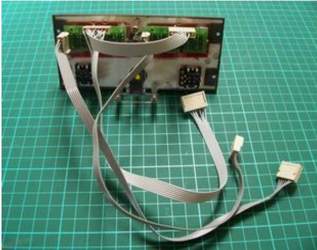
Your next major work is making up cables to connect your displays to your boards. I highly recommend making up multipin connectors. Don't try soldering directly to the display pins. Whatever method you end up using you will have a lot of pin connections to make, it's unavoidable!!
