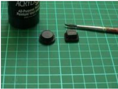
Here's the result. It will only take a few minutes using superglue. Edges need to be painted black to avoid light leakage when backlit. Use acrylic paint available from any craft shop.
