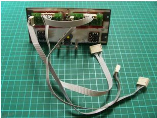
Your next major work is making up cables to connect your displays to your boards. I highly recommend making up multipin connectors. Don't try soldering directly to the display pins. Whatever method you end up using you will have a lot of pin connections to make, it's unavoidable!!
