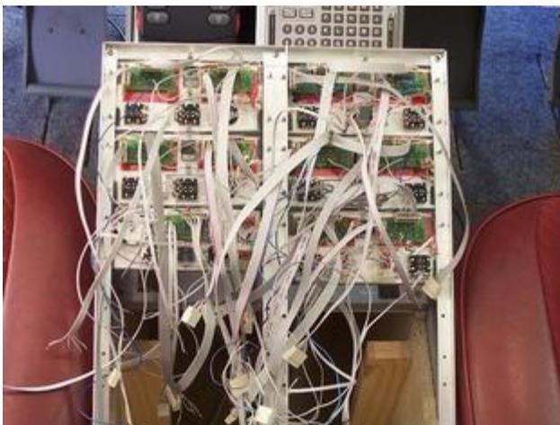
Here's an example of the final wiring mess for the full set of radios in the pedestal. It's really important therefore to take care making up cables to the length required and keeping good records of connections.
