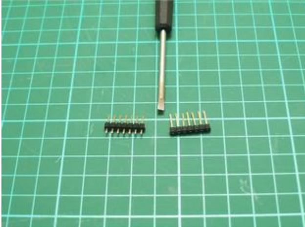
Standard pcb pins were used but due to the need to push them through from the underside I modified them by pushing the plastic support down to the base of the pins.
