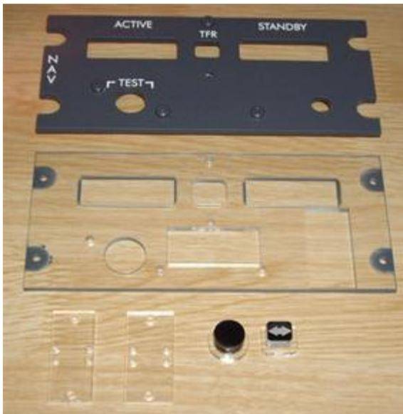
The NAV panel comprises a front plate laser cut and ready for backlighting, backplate, 2 x switch mounting plates and buttons.
