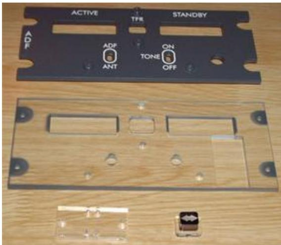
The ADF panel comprises a front plate laser cut and ready for backlighting, backplate, switch mounting plate and TFR button.
