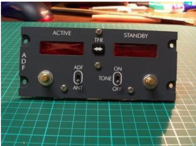
The completed hardware installation. For my ADF radio two encoders provide high and low digit selection. You may choose to use the more authentic dual concentric encoder or a single encoder with the encoder's pushbutton alternating between High & Low selection.
