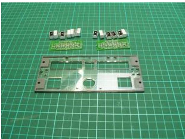
Now onto the construction of the 7-segment displays. Again always use the mounting PCB's. They only cost a few dollars each and make it a breeze to install.
