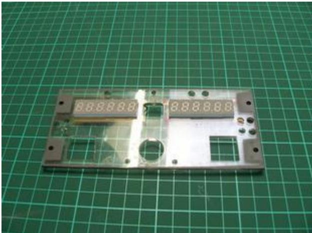
Place the displays onto the PCB's then mount the backplate over the displays prior to soldering. Turn the whole lot over and solder the displays onto the PCB's while mounted in the backplate. This will allow the displays to more easily insert through the backplate later on during final assembly. These backplates are laser cut to very fine tolerance and if you solder without doing this you'll end up needing to file the backplate holes to fit the displays. (Ask me how I know this!)
